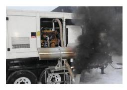
If you have a problem with smoke and odour from your diesel generator, the FOx module may be a perfect solution. The picture on the left shows a 100kW Tier 3 engine starting up without the FOx. On the
