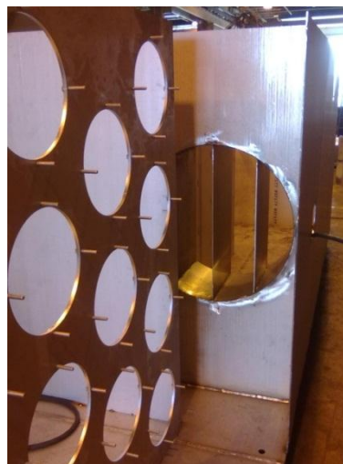
Bulkhead for FOx modules for 3MW engine
